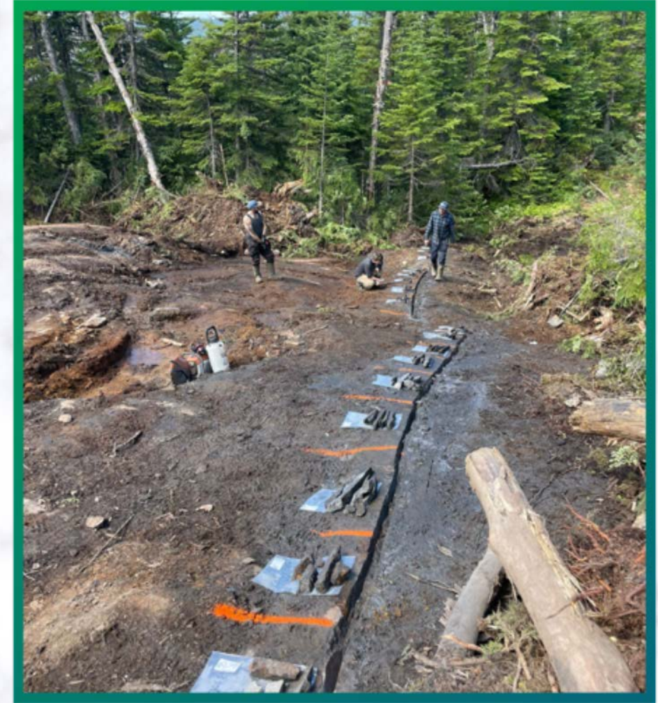
Graphite Outcrop Grading 17 - 45% Graphite being Channel sampled
